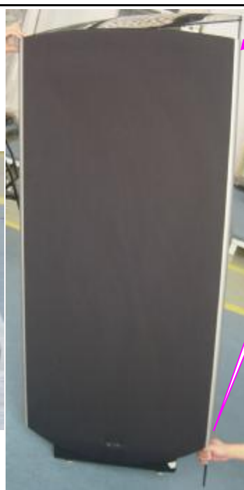
4. Use plastic curton rod to push the top plinth.
