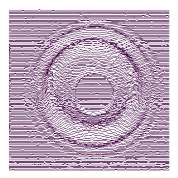
Figure 1. Laser scan of the midrange cone in the SP1415 Uni-Q driver array. The scan shows the motion of the cone at 3.1 kHz. Bending waves in the cone travel outwards from the coil to the surround where they are damped-out by the lossy surround material. This gentle 'ripple' effect is the ideal behaviour known as 'controlled breakup'.
