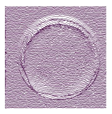
Figure 4. The first break-up mode in the SP1406 lower midrange unit is at 560Hz where the surround displays controlled resonance.
