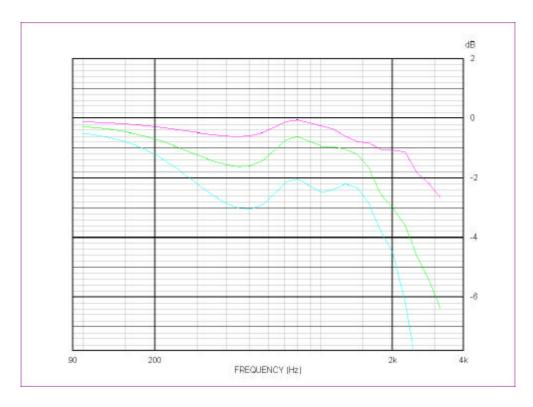
Figure 8. Off-axis response of a piston in R109 uni-Q cabinet. The curves are the acoustic pressure response at 15, 30 and 45 degrees horizontally off-axis, all relative to on-axis.
