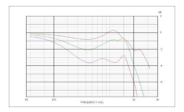
Figure 6. Off-axis response of a piston in a flat baffle, same dimensions as R109 uni-Q cabinet. The curves are the acoustic pressure response at 15, 30 and 45 degrees horizontally off-axis, all relative to on-axis.
