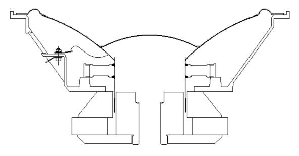
Figure 2. Cross-section of the new SP1405 Low Frequency Unit.
