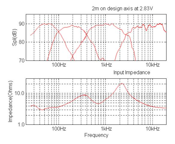
Figure 10. Individual unit responses and Input Impedance.
