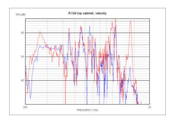
Figure 5. Comparison of the performance of braced and unbraced Uni-Q cabinets. The data is the velocity of front panel vibration due to excitation from the Uni-Q driver array. The braced cabinet (solid line) shows considerable improvement at 250Hz, 1kHz and 1.4kHz.
