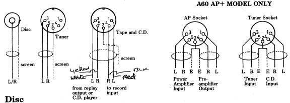
Your turntable lead should be fitted with two PHONO plugs wired as illustrated. If any other connector is fitted it should be removed and replaced by two PHONO plugs, or a high quality adaptor lead used to interface.
